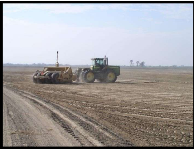
Figure 19. Land leveling as part CP to reduce sediment and nutrient losses ( http://www.la.nrcs.usda.gov )
